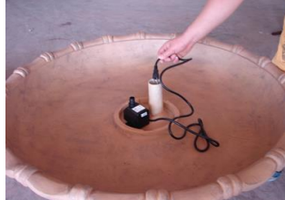
Get the wire of pump through plastic pipe of biggest plate center. Make sure the wire put into the biggest pedestal's cavity.
