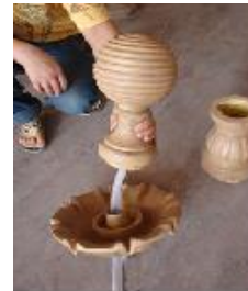
Feed the rubber hose through the plastic tube of smallest plate center. then connect top part and smallest plate tightly
