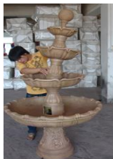
Feed the rubber hose through the plastic tube of second big plate then connect the small pillar and the second big plate tightly.
